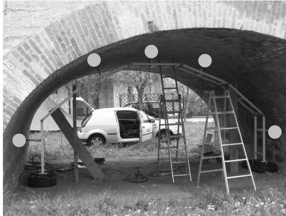
Figure 3 : Photograph of position of measuring points and special designed rack
