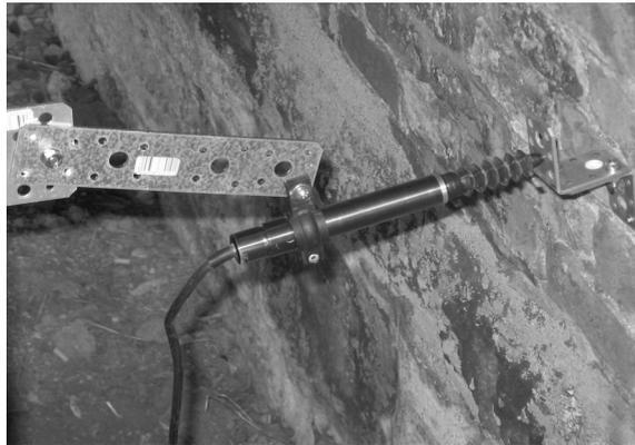
Figure 2 : Photograph of applied displacement transducer
