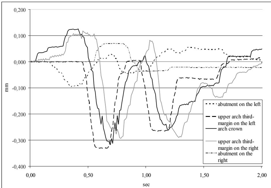
Figure 6 : Arch deflection due to 20 t axle locomotive at 60 km/h
