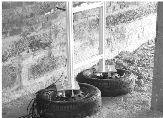
Figure 4 : Photograph of the developed mass-spring-system at the base of the framework
