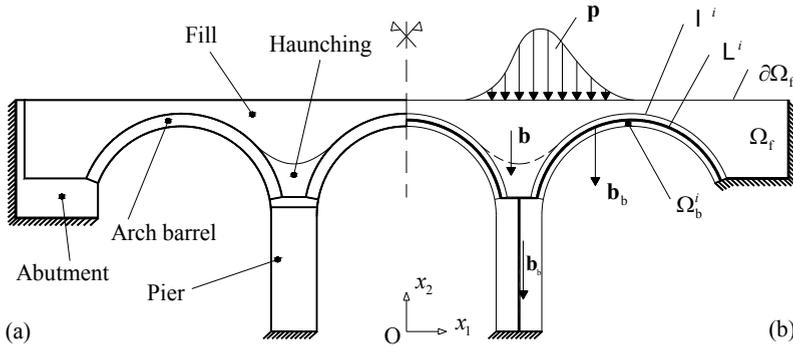
Fig. 1. (a) Longitudinal cross section and (b) two-dimensional model of the bridge.
