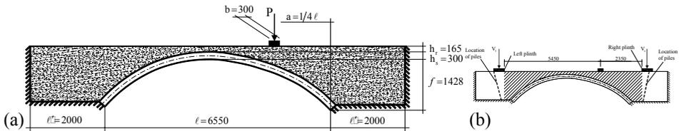
Fig. 3. (a) Prestwood bridge model (mm). (b) Position (mm) of the plinths of the loading system and of the piles at abutments.
