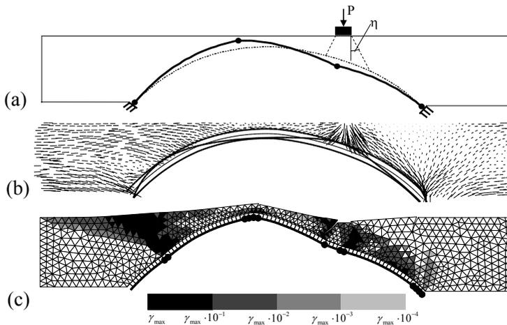
Fig. 4. (a) Collapse mechanism with non resistant fill ( $P_{nrf} = 46.2\text{kN}$ ); (b) in-plane principal stress field and line of thrust (plane strain fill) ( $P_{strain}^{lb} = 208.8\text{kN}$ ); (c) collapse mechanism and contour plot of the maximum shear strain rate from compatible model (plane strain fill) ( $P_{strain}^{ub} = 254.5\text{kN}$ ).
