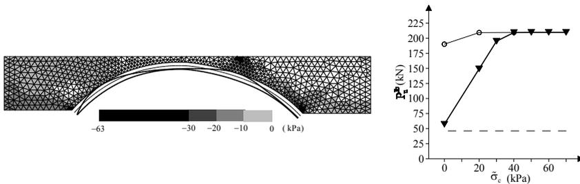
Fig. 5. (a) Contour plot of the minimum compressive stress  $\sigma_3$ . (b) Influence of the allowable transverse stress  $\bar{\sigma}_c$  on the lower estimates of collapse load (bold line); estimates obtained by imposing plain strain under the punch (thin line); estimates obtained by assuming heavy non resistant fill (dashed line).
