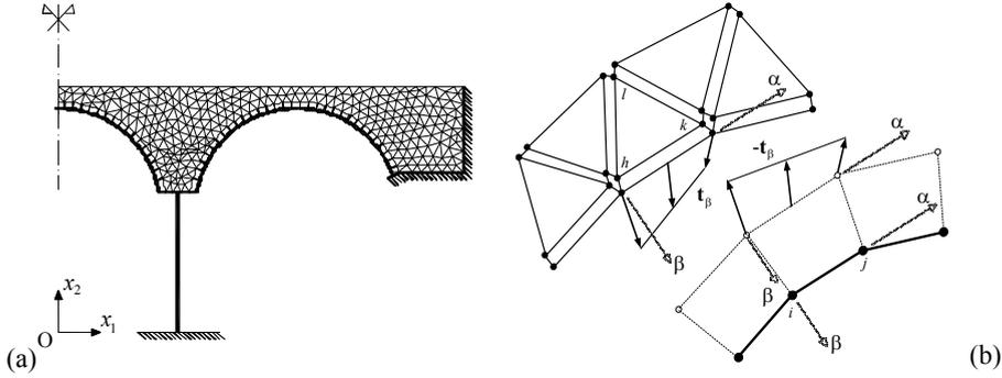
Fig. 2. (a) Finite element model of the bridge; (b) the finite element equilibrium model: arch-fill interaction tractions.
