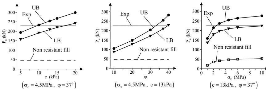
Fig. 6. Effects (a) of the cohesion  $c$ , (b) of the angle of internal friction  $\phi$  and (c) of masonry compressive strength  $\sigma_c$ .
