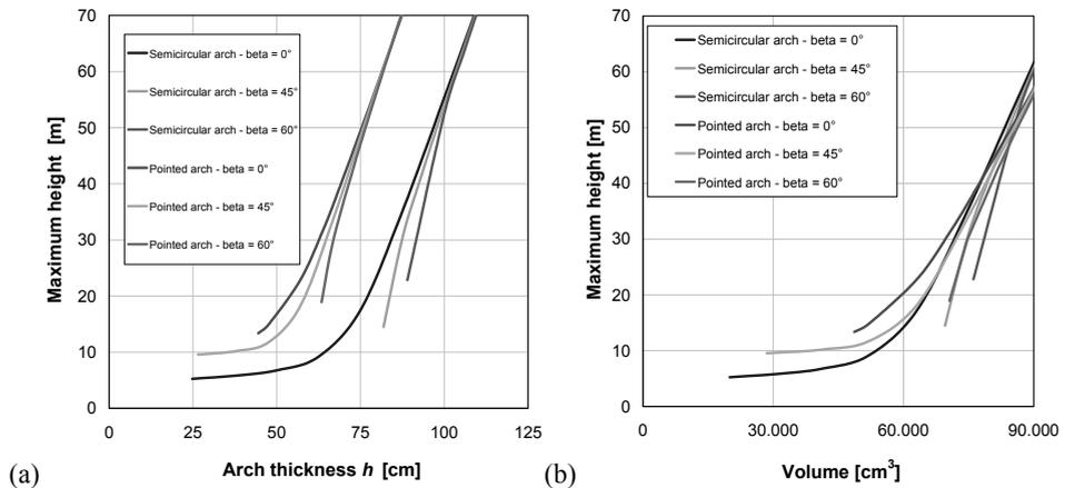
Figure 8. Maximum height of the arch-wall system versus arch thickness  $h$  (left) and versus volume of the arch (right).
