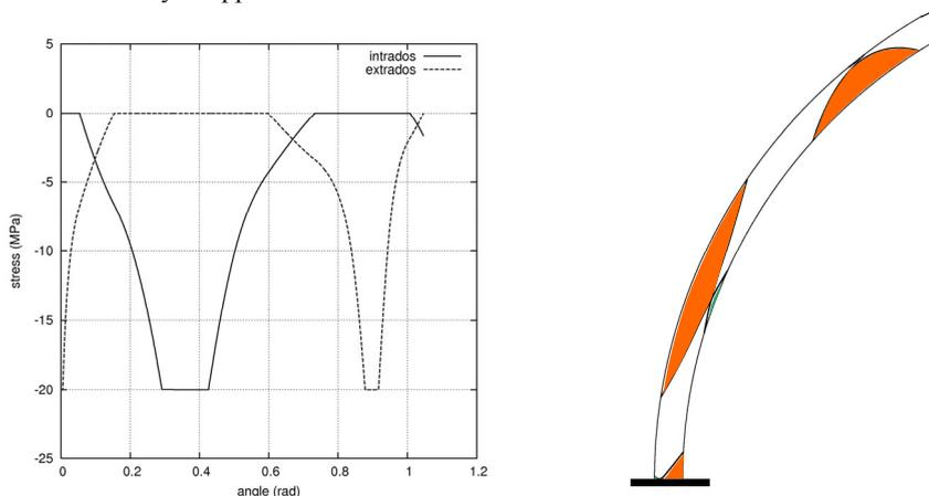
Figure 11. Extrados and intrados stresses (left) and extension of the non-linear regions along the left half of the arch (right).
