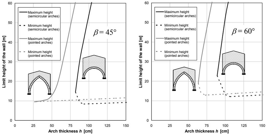
Figure 7. Limit height of the arch-wall system for a semicircular and a pointed arch (left:  $\beta = 45^\circ$ ; right:  $\beta = 60^\circ$ ).
