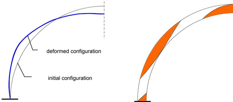
Figure 9. Left: deformed configuration (displacement magnified two times); right: non-linear regions under tension (in orange).
