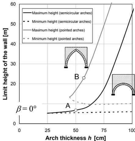
Figure 6. Limit height of the arch-wall system for a semicircular and a pointed arch ( $\beta = 0^\circ$ ).
