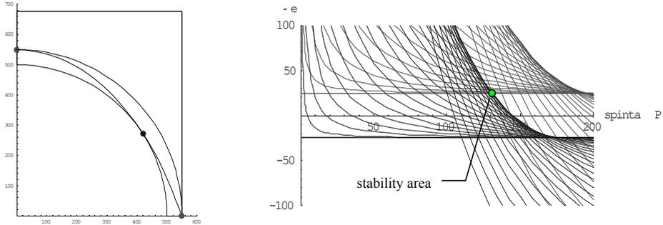
Figure 5 a, b. Line of thrust and stability area (semicircular arch;  $\beta = 0^\circ$ ,  $h = 50$  cm).
