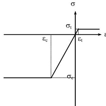
Figure 3. Non-linear stress-strain relation.
