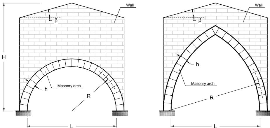
Figure 1. Scheme of the arch-wall system for semicircular (left) and pointed (right) arches.
