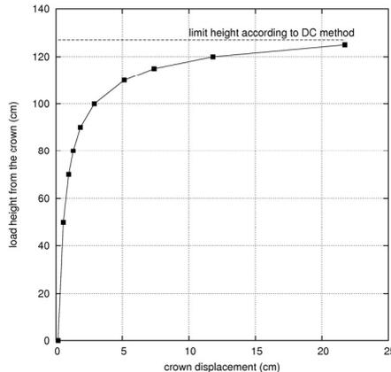
Figure 10. Plot of the crown vertical displacement for different values of the wall height.
