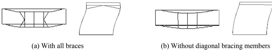
Figure 8: Buckling mode during filling concrete into steel tubes of arch rib
