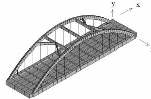
Figure 3 : Space Finite Element Model
