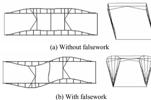
Figure 9 : Buckling mode during installation of cross beam
