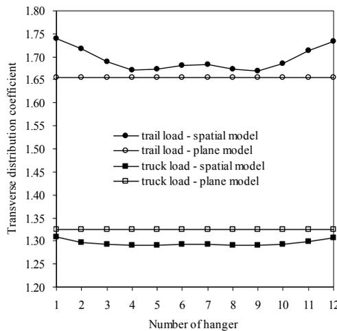
Figure 4: Transversely distribution coefficients of live load
