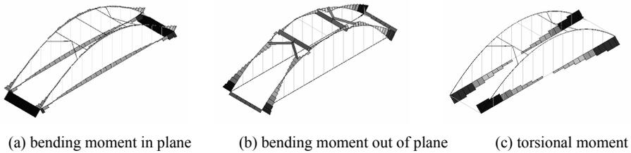
Figure 5: Internal force when erecting cross beam
