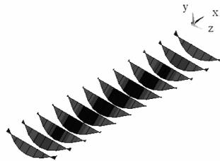
Figure 6 : Bending moment of deck cross beams under dead load
