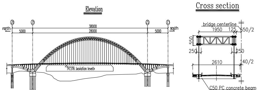
Figure 1 : General layout of the bridge (unit: cm )
