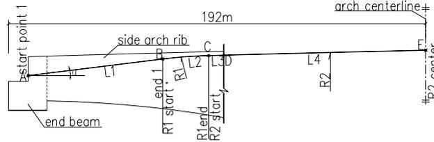
Figure 3: The computing diagram for the prestress loss of the tie bar strand
