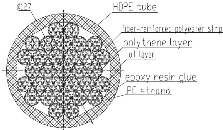
Figure 2: The tie bar cross-sectional diagram
