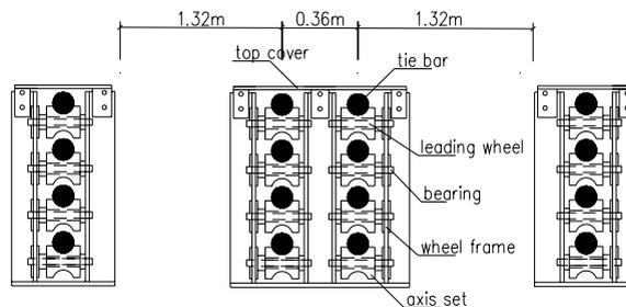
Figure 4: Diagram for a leading wheel frame
