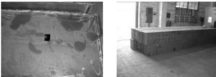
Fig.12: Model experiment of the deck slab under negative moment
