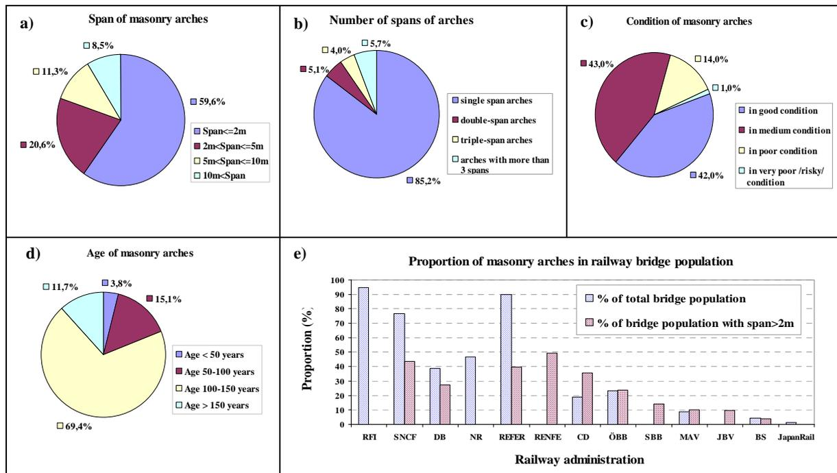
Figure 1: Statistical distribution of masonry arch bridges according to their a) span length b) span number c) condition d) age.
