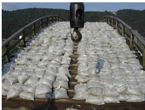
Figure 13: Uniform load of 60 tons
