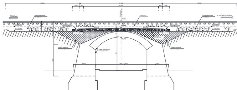
Figure 4: Reconstruction of arch bridge – longitudinal section
