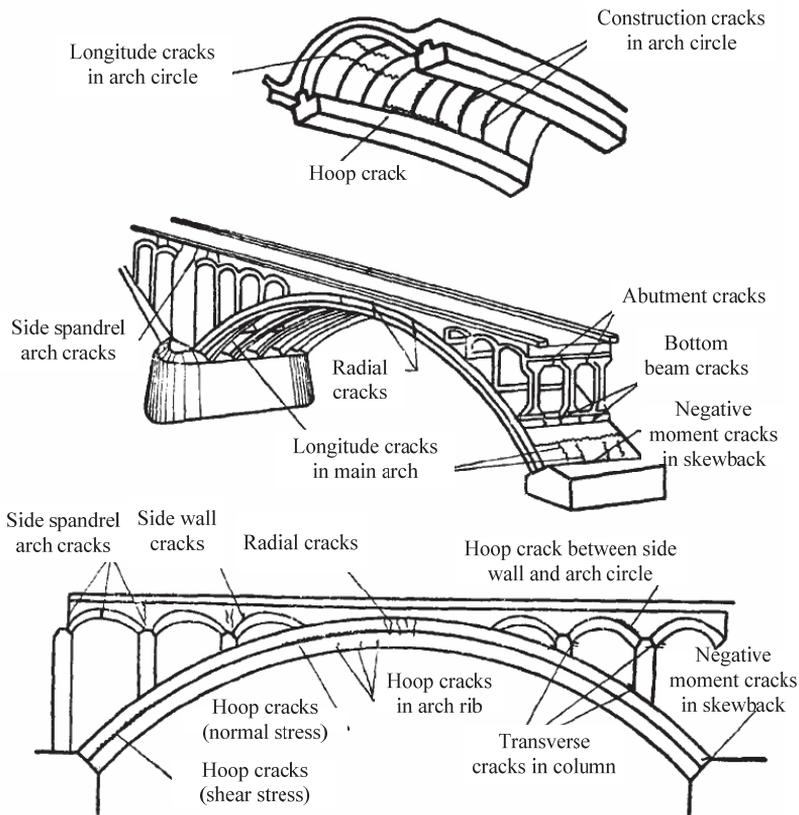
Figure 1: Double-curved arch bridge cracks
