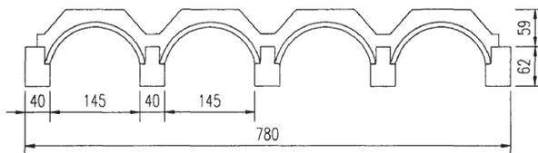
Figure 5: Transverse section of Shuiwen Bridge (dimensions in cm)
