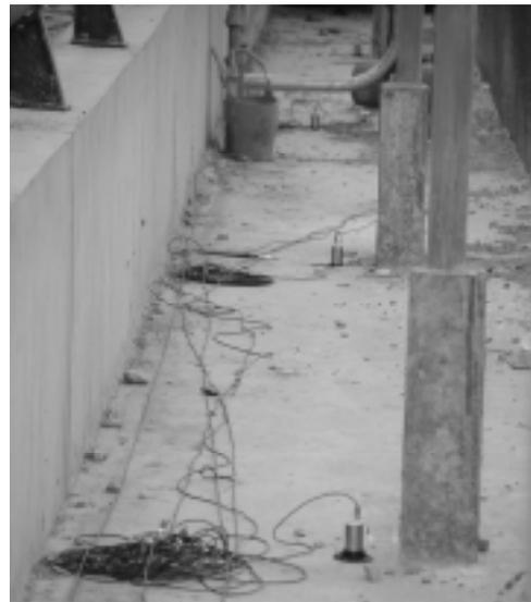
Figure 3: Accelerometers mounted on bridge deck
