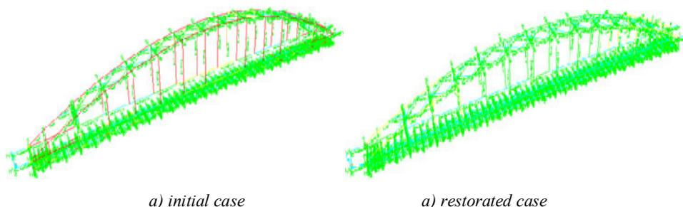
**Fig. 11.** The design check results for initial and restored cases.
