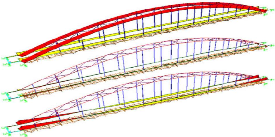
*Fig. 10. Maximum internal forces for dead, moving and wind load case.*
