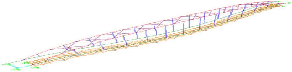
*Fig. 9. Maximum displacements for dead, moving and wind load case.*
