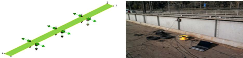
Fig. 5. The accelerometers location and placements in the bridge.
