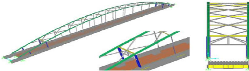
*Fig. 7. The initial finite element model of the bridge.*
