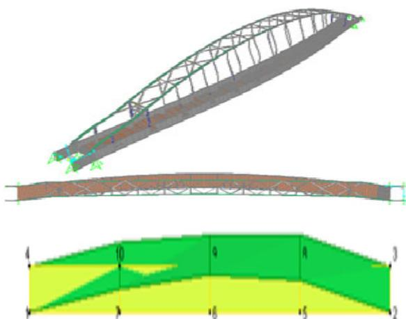
*Fig. 8. The first analytical (top) and experimental (bottom) mode shapes of the bridge.*
