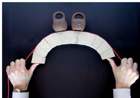
*Fig. 3. Schematic functioning of "reinforced arch method". The ashlars are compressed according to the amount of tensioning given to the rope.*
