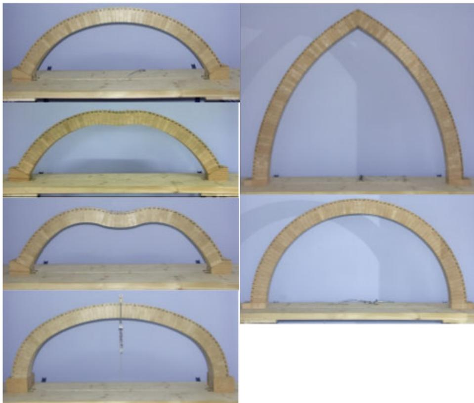
**Fig. 8.** The six geometries of the models tested under concentrated vertical load. From the top: circular, ribbed, ribbed+small depression, ribbed+large depression, polycentric and gothic. (Jurina - Giglio, 2008).
