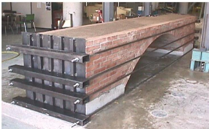
**Fig. 2.** Steel plates confining the infill and the ties balancing the plates.
