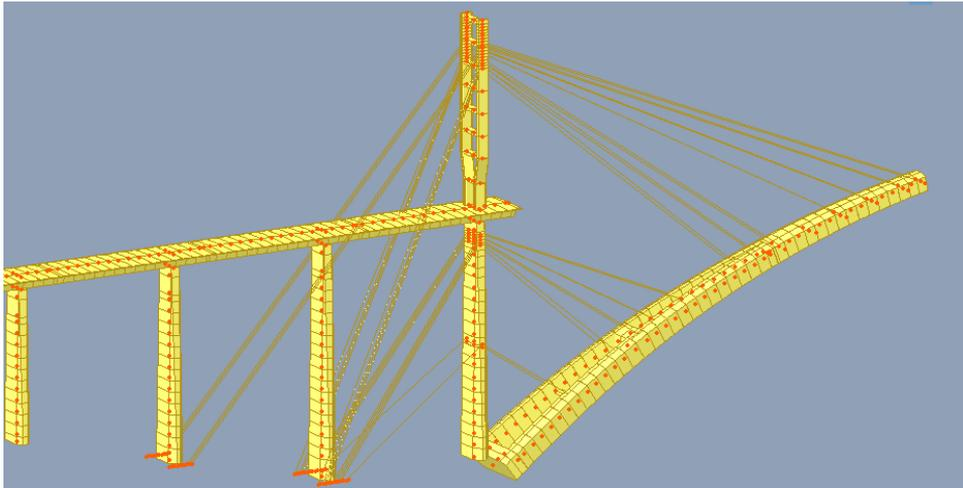
*Fig. 4. Close-up view of an intermediate stage of the construction process.*
