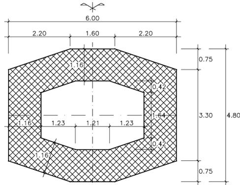
*Fig. 2. Typical cross section of the arch. Relationship between depth and chamfers.*
