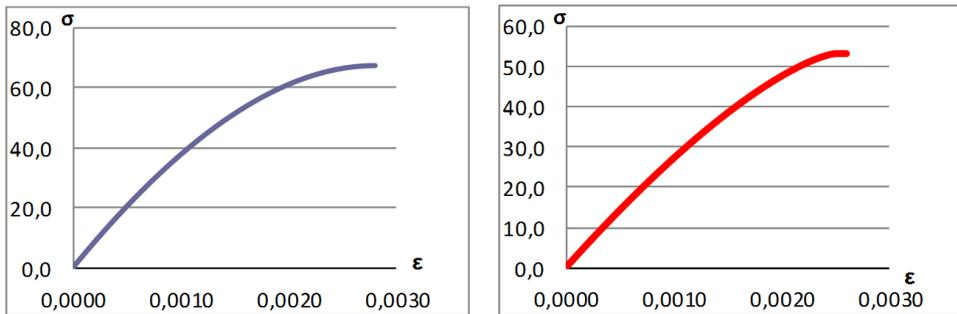
*Fig. 8.  $\sigma$ - $\epsilon$  diagrams of concrete HA-80 for the sectional nonlinear calculation.*
