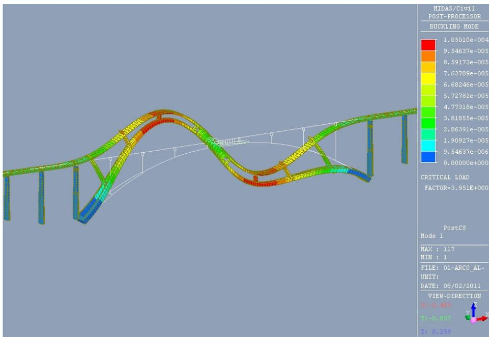
Fig. 6. Buckling mode corresponding to the hypothesis called S08 – Min.
