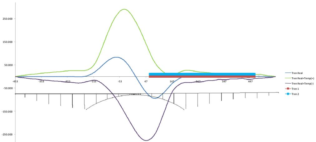
*Fig. 9. Deformed deck for a specific case of two HSML trains at 300 km/h.*
