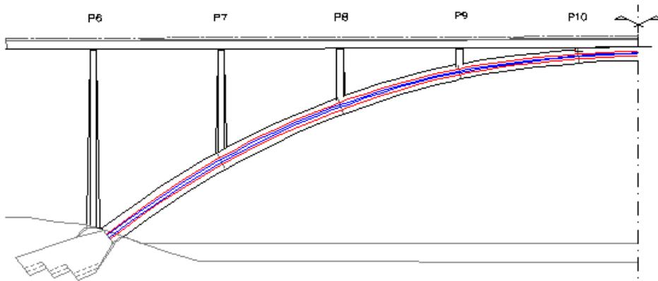
*Fig. 1. Pressure lines (blue) in central area (red) of the cross section is the key of the design.*
