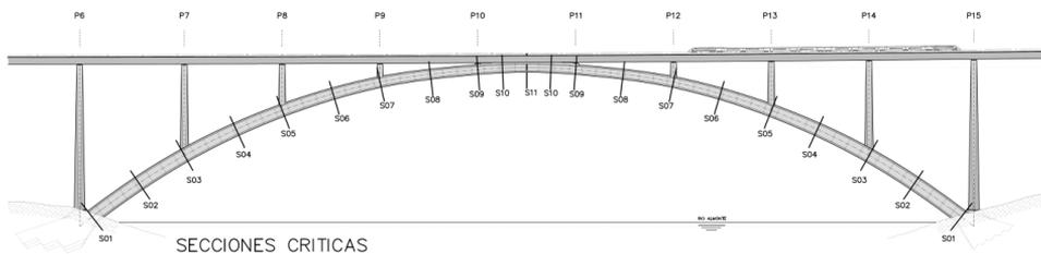
*Fig. 5. Study of critical sections.*
