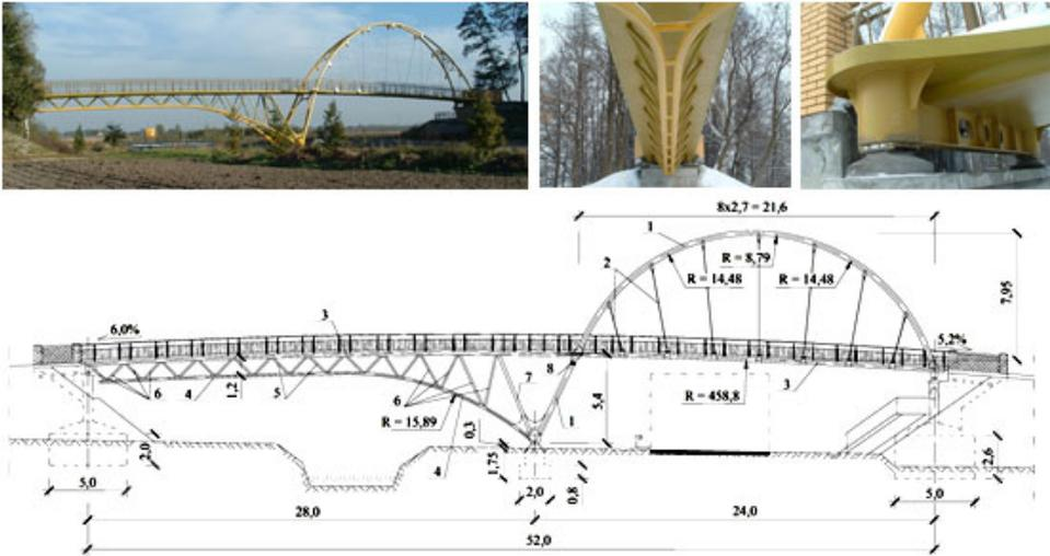
**Fig. 3.** Arch footbridge in Bieruń Stary, Poland (Engineering Studio Project s.c.): 1 – steel tube  $\varnothing 244.5/8$  mm; 2 – steel bar  $\varnothing 30$  mm; 3 – steel box-girder filled with concrete (steel plate 6 mm thick); 4 – steel tube  $\varnothing 193.7/14.2$  mm; 5 – steel tube  $\varnothing 101.6/7.1$  mm; 6 – steel tube  $\varnothing 108.0/8.0$  mm; 7 – steel tube  $\varnothing 168.3/12.5$  mm; 8 – hinged connection constructed using elastomeric bearing placed in steel tubes.
