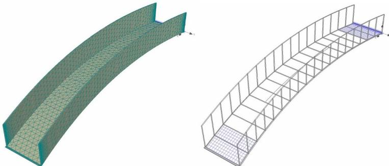
Fig. 5. Finite element mesh on the left and on the right: Segmentation of macroelements to surfaces and reinforcement of the anchoring area.
