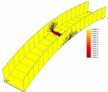
**Fig. 7.** Cracks on the structure prior to the failure, the applied force of  $18.9 \text{ kN/m}^2$ , the maximum crack width  $3.18 \text{ mm}$ .
