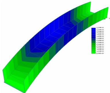
**Fig. 6.** Vertical deflection of the structure before failure, the applied force of  $18.9 \text{ kN/m}^2$ , the maximum deflection value  $-22.59 \text{ mm}$ .
