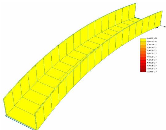
**Fig. 9.** Cracks on the structure, the applied force of  $4,2 \text{ kN/m}^2$ , the maximum crack width  $0,0006 \text{ mm}$ .
