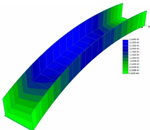
**Fig. 8.** Vertical deflection of the structure, the applied force of  $4,2 \text{ kN/m}^2$ , the maximum deflection value  $-2.66 \text{ mm}$ .
