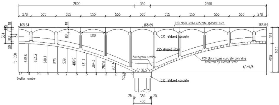
**Fig. 4.** All open spandrel light stone arch, Guanyin Bridge.
