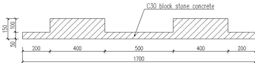
*Fig. 3. Cross-section of main arch ring, Guanyin Bridge.*
