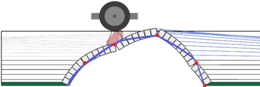
*Fig. 7. Collapse mechanism foreseen by RING.*
