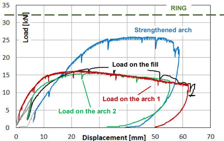
Fig. 6. Load-displacement diagrams for the other models [16] and for the RING model.
