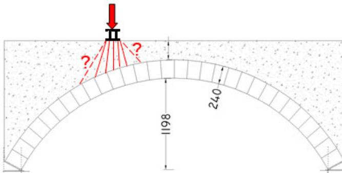
*Fig. 4. Loading on the fill surface (test n. 3).*
