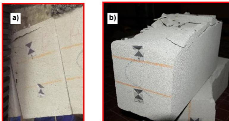
*Fig. 8. Plastic hinge located just below the load (fig.s 6 and 7):
