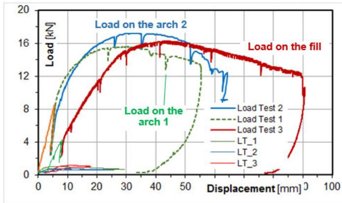
**Fig. 5.** Load-Displacement diagrams for the three tests. Thin lines: bare arches. Bold lines: arches + fill. Tests 1 and 2: load applied on the arch extrados; test 3: load applied on the fill surface.
