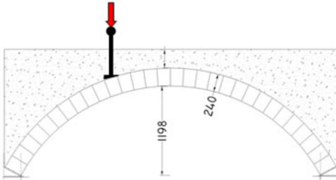
*Fig. 3. Loading directly on the arch (tests 1 and 2).*
