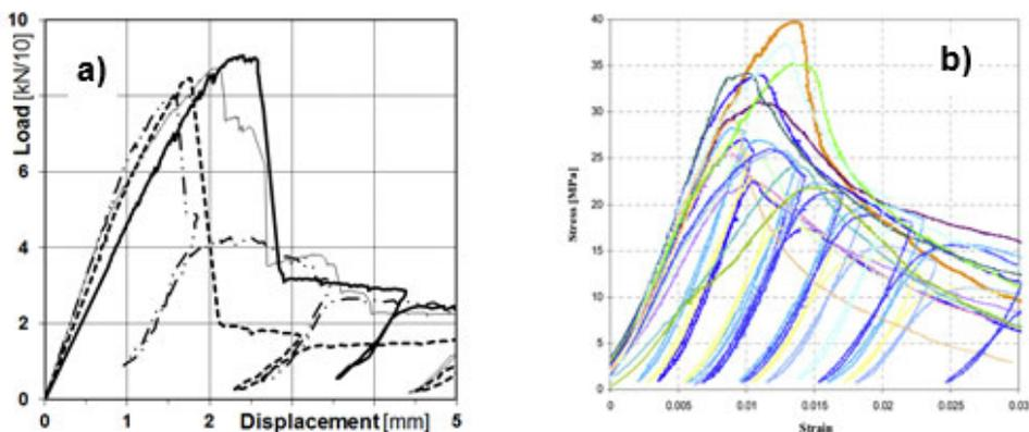
**Fig. 1.** Compressive response of a) aerated autoclaved concrete; b) solid clay brickwork [9] (note that the specimens were prisms with different dimensions  $\Rightarrow$  different loads).
