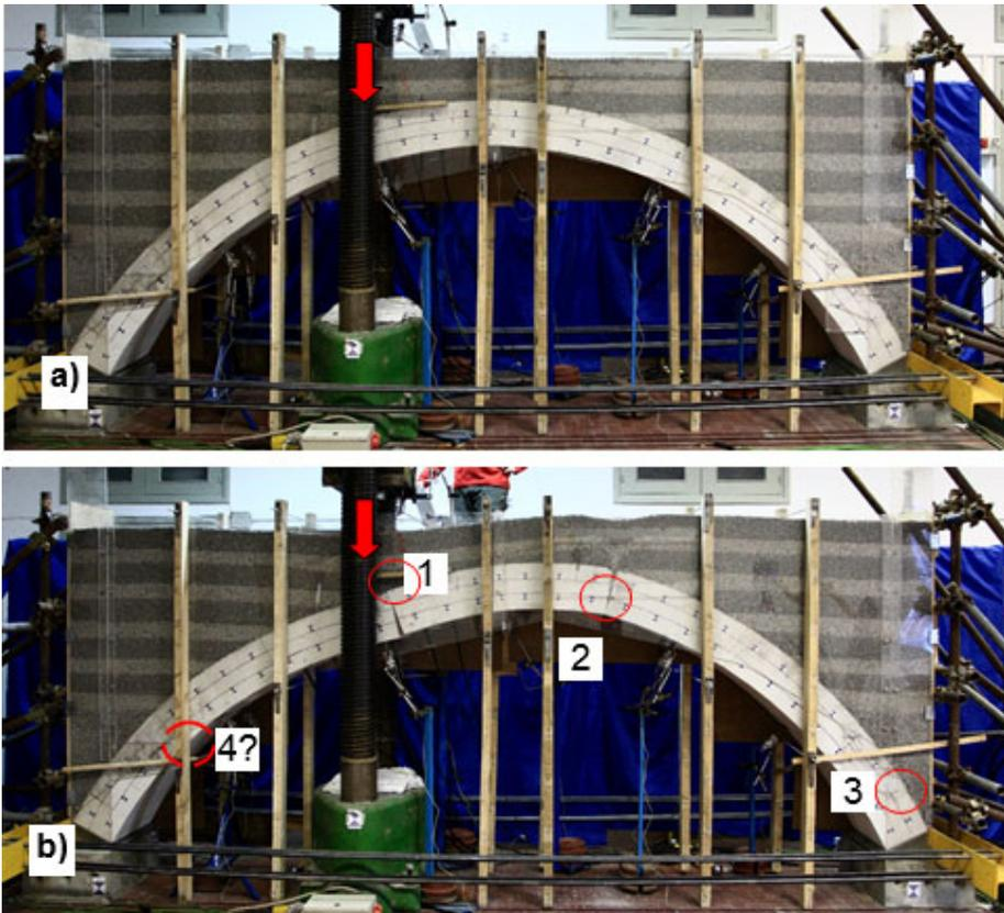
*Fig. 6. Model 3. a) unloaded; b) at maximum displacement (90 mm). Red circles stand for the detected hinges.*
