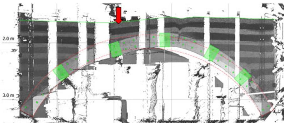
*Fig. 7. Deformed shape of the arch at the maximum displacement (90mm) compared to the undeformed shape.*
