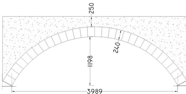
**Fig. 2.** Arch geometry. The arch thickness (third dimension) is 450mm.
