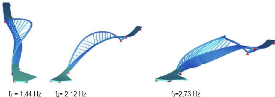
**Fig. 4.** Eigenforms and frequencies after redesign of superstructure.
