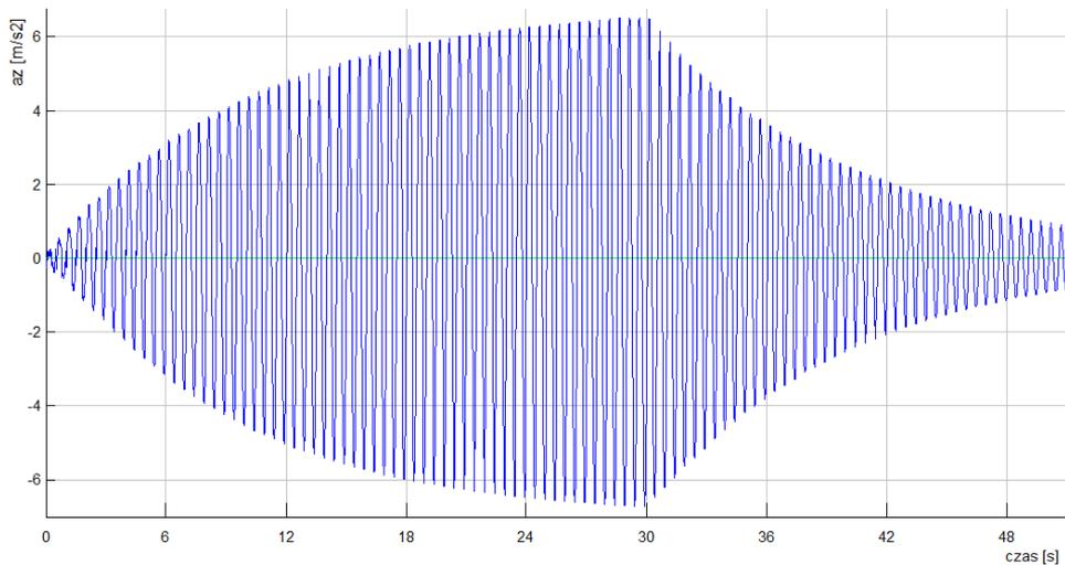
**Fig. 6.** Max. vertical acceleration on deck – test C5 – max=6.515 [m/s<sup>2</sup>].
