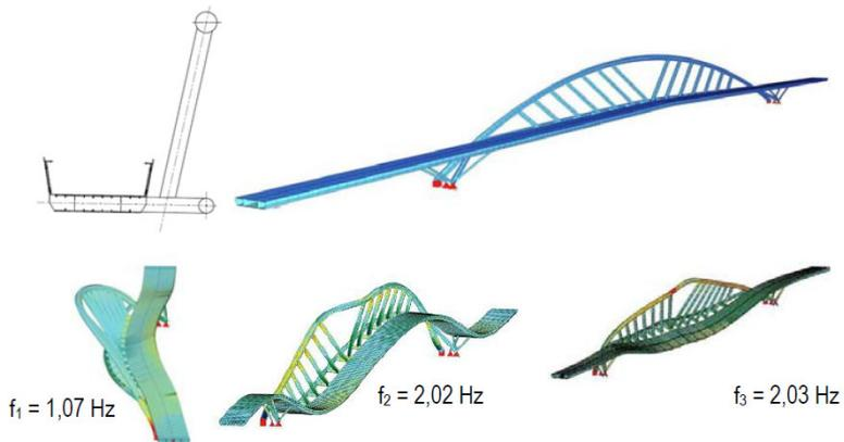
*Fig. 2. Original FEM SOFiSTiK model, cross section and first three eigen forms and frequencies.*
