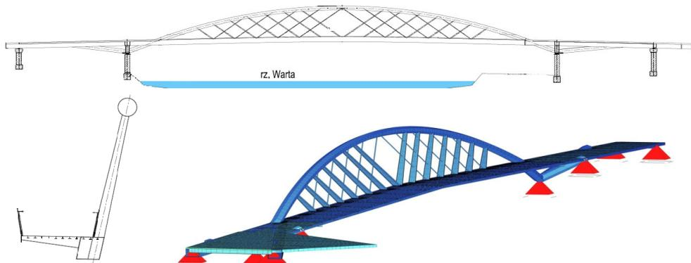
**Fig. 3.** Modified design. Elevation, cross section and FEM SOFiSTiK model.
