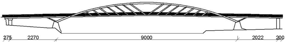
*Fig. 1. The architectural vision and side view of the footbridge. Design: MOST Świdzki [3].*
