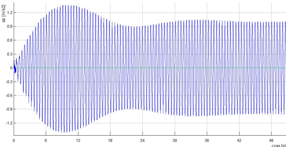
Fig. 5. Test Pf3 max. vertical acceleration of the deck – stabilization  $\sim 1$  [m/s<sup>2</sup>].
