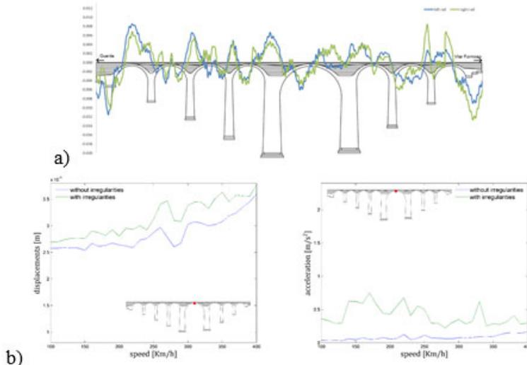
**Fig. 4.** Numerical results: a) Longitudinal levelling profiles of the left and right rail of the C $\hat{o}$ a bridge; b) Vertical response at the centre of principal arch A5 in terms of displacements and accelerations.
