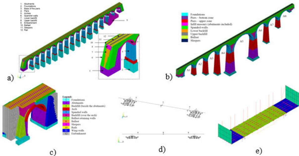
**Fig. 2.** FE global models: a) Durrães bridge; b) Cóa bridge; c) PK 124 bridge; d) Alfa Pendular train; e) Freight train.
