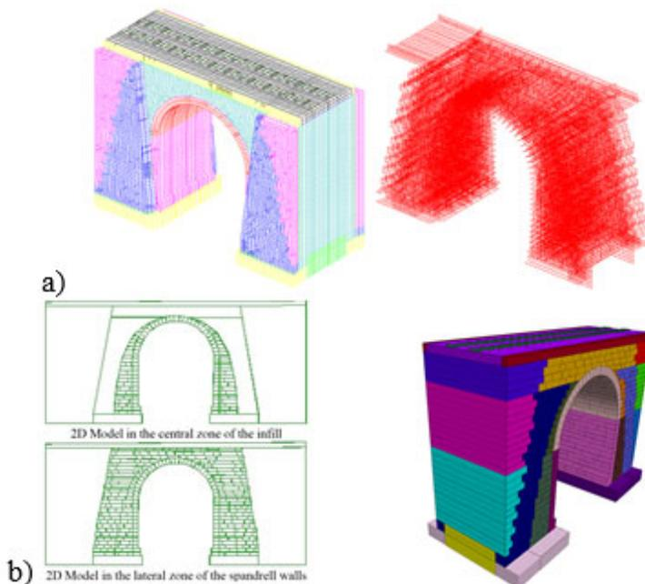
*Fig. 3. FE and DE detailed models of PK 124 bridge: a) FEM based CAST3M model (solid and joint elements); b) DEM based 2D and 3D models.*
