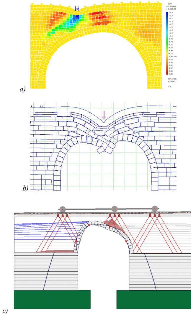
**Fig. 6.** FE and DE detailed models of PK 124 bridge: a) FEM based CAST3M model; b) DEM based UDEC model; c) RB based RING model.
