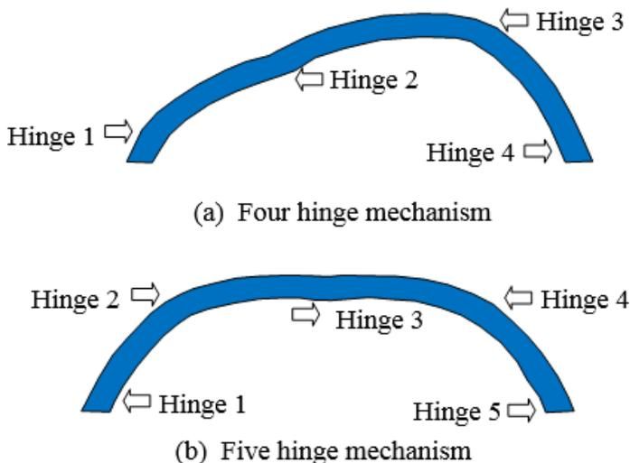
*Fig. 4. Failure mechanism of the masonry arch.*
