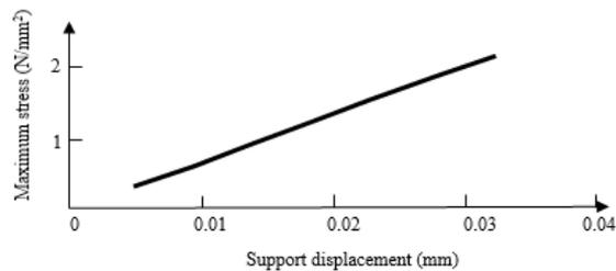
Fig. 2. Maximum principal stress due to support displacement [3].
