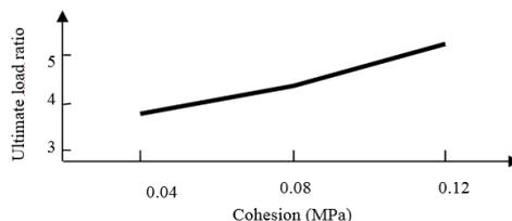
*Fig. 3. Maxi Ultimate load vs. cohesion of backfill ( $\phi=30^\circ$ ) [24].*
