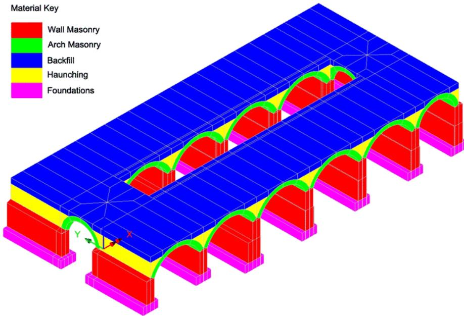
*Fig. 1. Masonry arch bridge modelled in FE software [1].*
