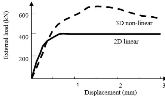
Fig. 5. Load deformation response of single span bridge [16].
