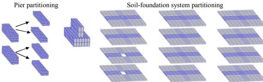
*Fig. 4. Substructure partitioning.*
