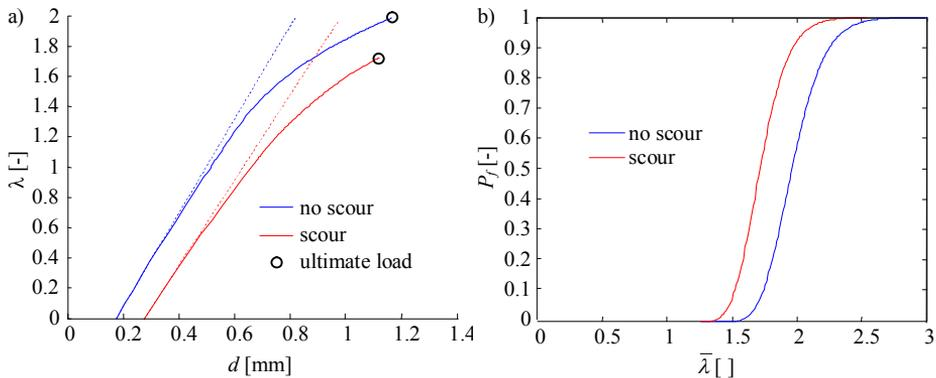
**Fig. 6.** Load multiplier vs. midspan vertical displacement curve (a), and probability of collapse vs. mean load multiplier  $\bar{\lambda}$  (b) for the cases corresponding to no scour and scour depth  $s=1.2\text{m}$ .
