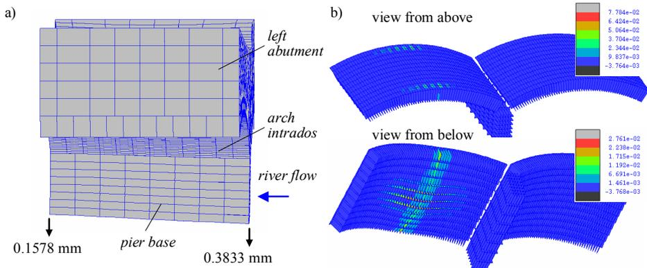
**Fig. 5.** a) Deformed shape after scouring action ( $s = 1.2\text{m}$ ), b) plastic work of the tensile and shear stresses.
