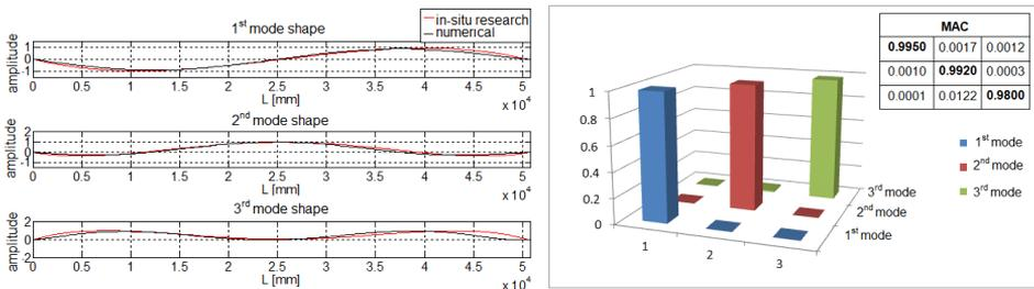
Fig. 9. The course of compared mode shapes for the facility and matrix MAC [6].
