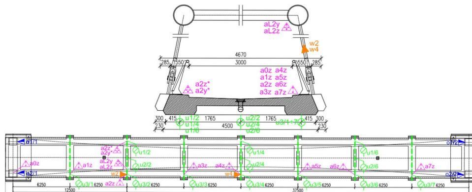
Fig. 2. Location of measuring points [7].
