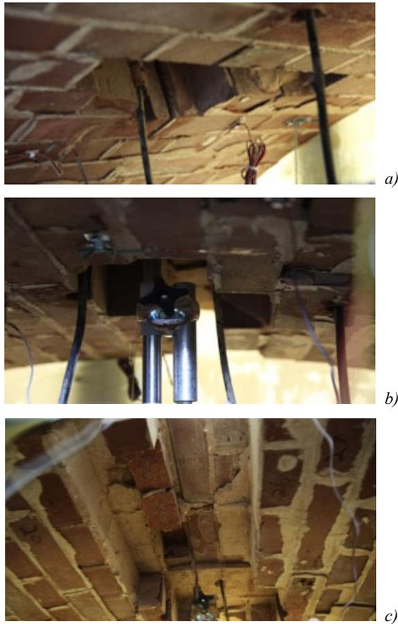
**Fig. 7.** Lost bricks at: a) state 1, b) state 2, and c) state 3 and 4.
