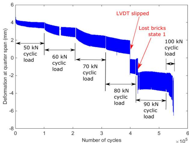
**Fig. 4.** Increase of displacement amplitude at the quarter span against number of cycles –EP5.
