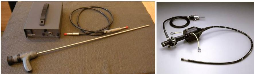
Fig. 2. Endoscope for technical (left) and medical (right) tests [www.optyczne.pl].
