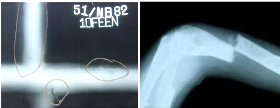
*Fig. 7. Conventional radiological tests: defects of welds in steel bridge arch (left) and broken bone (right) [www.zsm.com.pl].*
