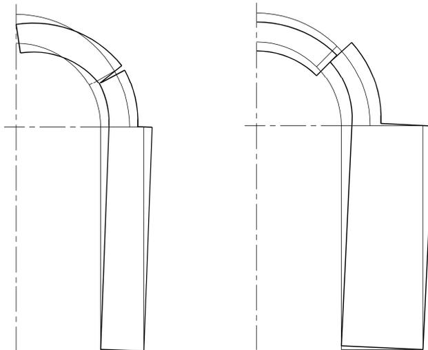
**Fig. 6.** Rotational collapse mode (left) and mixed collapse mode "à la De La Hire" (right).
