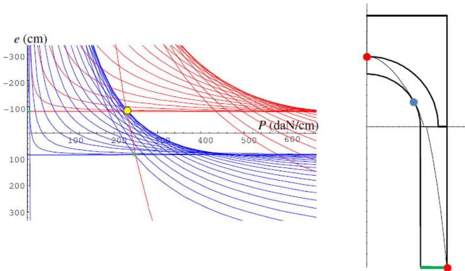
**Fig. 4.** Area of stability (left) and corresponding thrust line (right) for a limit thickness of the piers  $B_{lim} = 2.54$  m.
