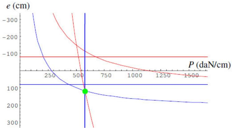
**Fig. 5.** Area of stability for the limit thickness of the piers  $B_{DLH} = 4.93$  m, assuming the mechanical model proposed by De La Hire.
