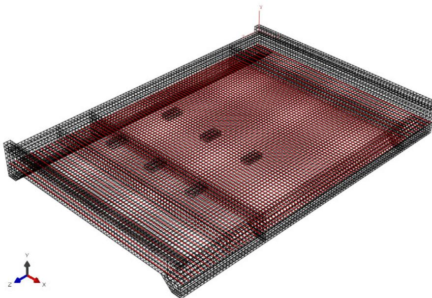
*Fig. 4. 3D Finite Element Model of one span of the bridge.*
