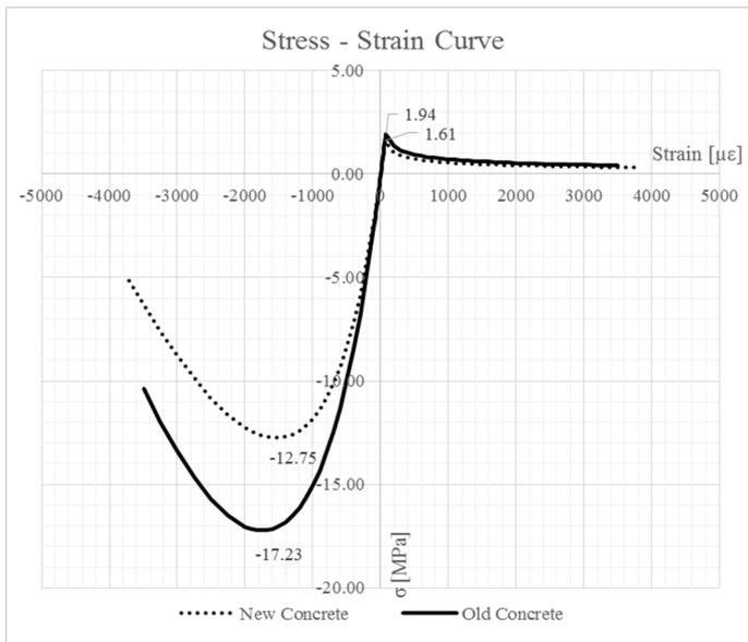
Fig. 3. Stress-Strain curve for New and Old concrete (1MPa=145psi).
